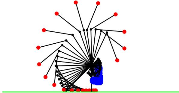
Fig. 2. The motion of the trebuchet at constant time intervals.
