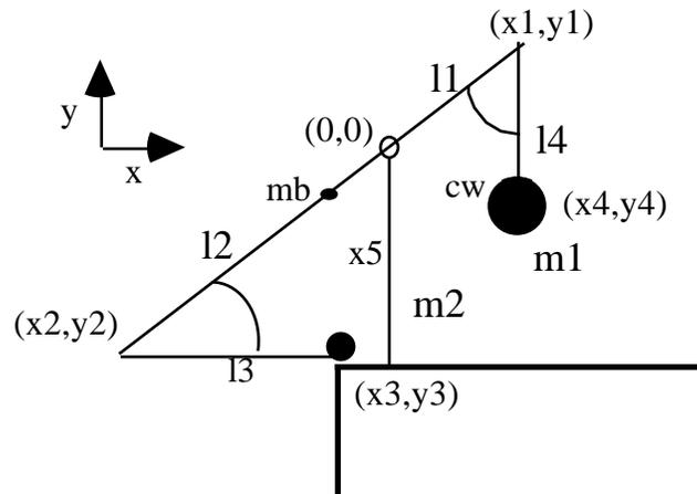
Fig. 6. The trebuchet with an unconstrained sling.
